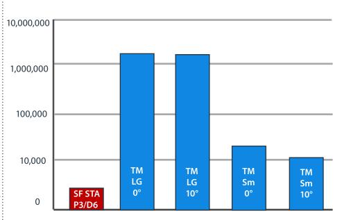
Number of cycles survived at a Load of 228 N. \*Data on file at Arthrosurface
